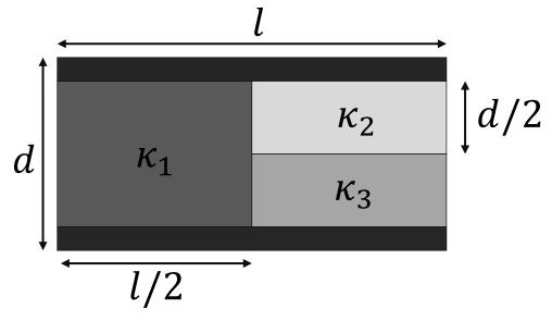
Q1: Find the capacitance of each capacitor after adding the dielectrics, as shown in the figure.
